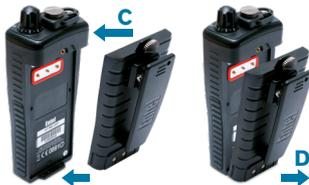
1. To attach, locate the pegs on the bottom of the battery into the slots on the radio and press the top of the battery against the radio. Secure battery by tightening the screw clockwise by hand. (Do not use any implement or over tighten) (C).
